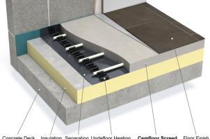
Concrete Deck Insulation Separating Undefloor Heating Cemfloor Screed Floor Finish Membrane
